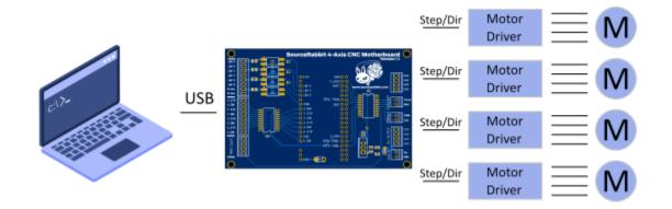
The 4-Axis CNC Motherboard is a "small computer" that connects a personal computer with **stepper and servo drivers** operating with **Step/Direction** pulses. It is compatible with all motor controllers on the market, can produce **120,000 pulses per second** and is intended for controlling 3 or 4 Axis CNC machine tools such as Router, Mills, Plasma and Lasers cutters.
